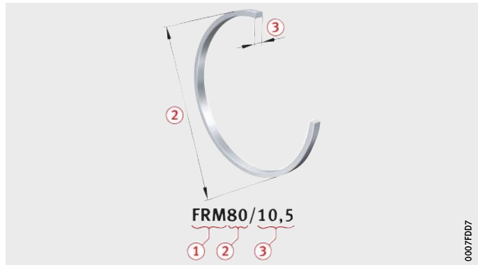
Figure 9 Designation structure of locating rings, example
